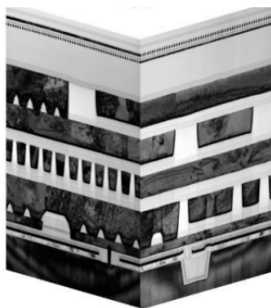
Figures: (Left) Cross-sectional TEM image of 16-nm half-pitch cross-point Selector-Only-Memory with periphery under cell architecture (Right) Cycle endurance characteristics of measured raw bit error rate with write cycles.
